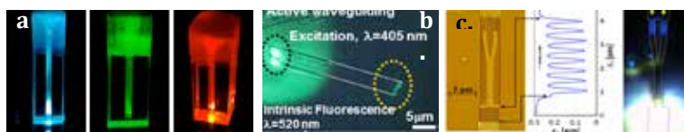
Figure 1. a. Multicolor visible FFF-Nanodots; b. Active waveguiding in peptide tape; c. Peptide 1x2-power Y-optical splitter with grating couplers at all three ports
